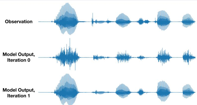
We qualitatively demonstrate AVF on modeling the TIMIT speech data set. At the initial inference iteration of each step, the model outputs a *prediction* of the observation. At subsequent inference iterations, the output *reconstruction* is refined using approximate posterior gradients.
