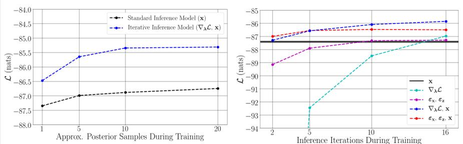
**Iterative inference models quantitatively outperform standard inference models with identical architectures** on MNIST (*nats*) and CIFAR-10 (*bits/dim*) (left). Iterative inference models **converge to similar approximate posterior estimates significantly faster than Variational EM** (right).
